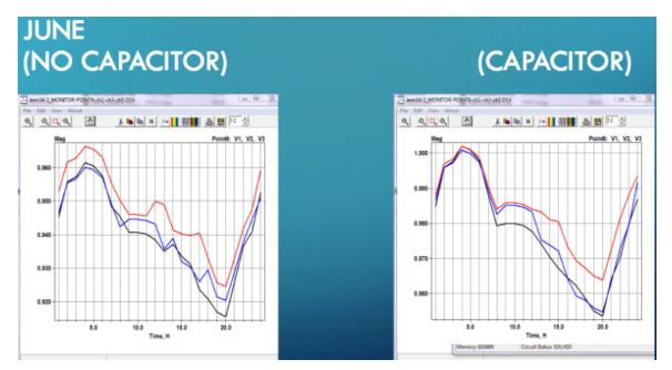
The graph below describes how regulator taps change over a period of 24 hours for the month of June. We analyzed for December as well and noticed how the regulator was reacting to different loads.
